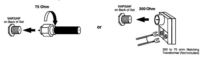
**Cable Connection** – For reception of cable channels, connect the cable supplied by your local cable company. **In the SETUP menu, set the MODE to CABLE.** (Refer to Antenna Mode section.)
